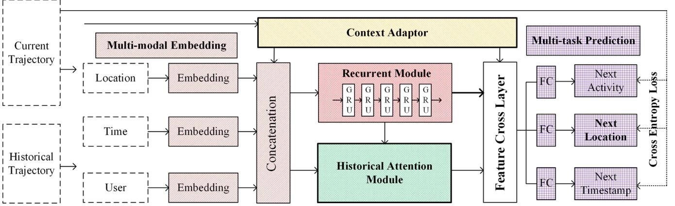
Fig. 3: The main architecture of DeepMove, which contains three major parts: 1) multi-modal embedding module for raw feature extracting; 2) recurrent module and historical attention module for sequential modelling; 3) context adaptor and multi-task prediction output for semantic modelling.
